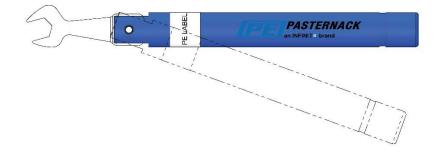
Torque wrench handle will break over when preset torque is achieved. Take note of the wrench bit orientation relative to the direction of motion/rotation.
