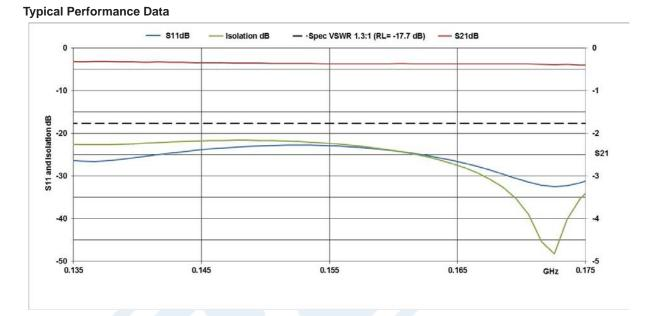
High Power Circulator With 20 dB Isolation From 135 MHz to 175 MHz, 150 Watts And N Female from Pasternack Enterprises has same day shipment for domestic and International orders. Our RF, microwave and millimeter wave products maintain a 99% availability and are part of the broadest selection in the industry.
